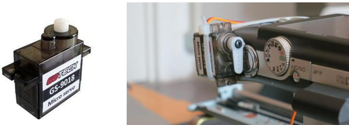
Figure 3: The servo motor connected to the camera.
