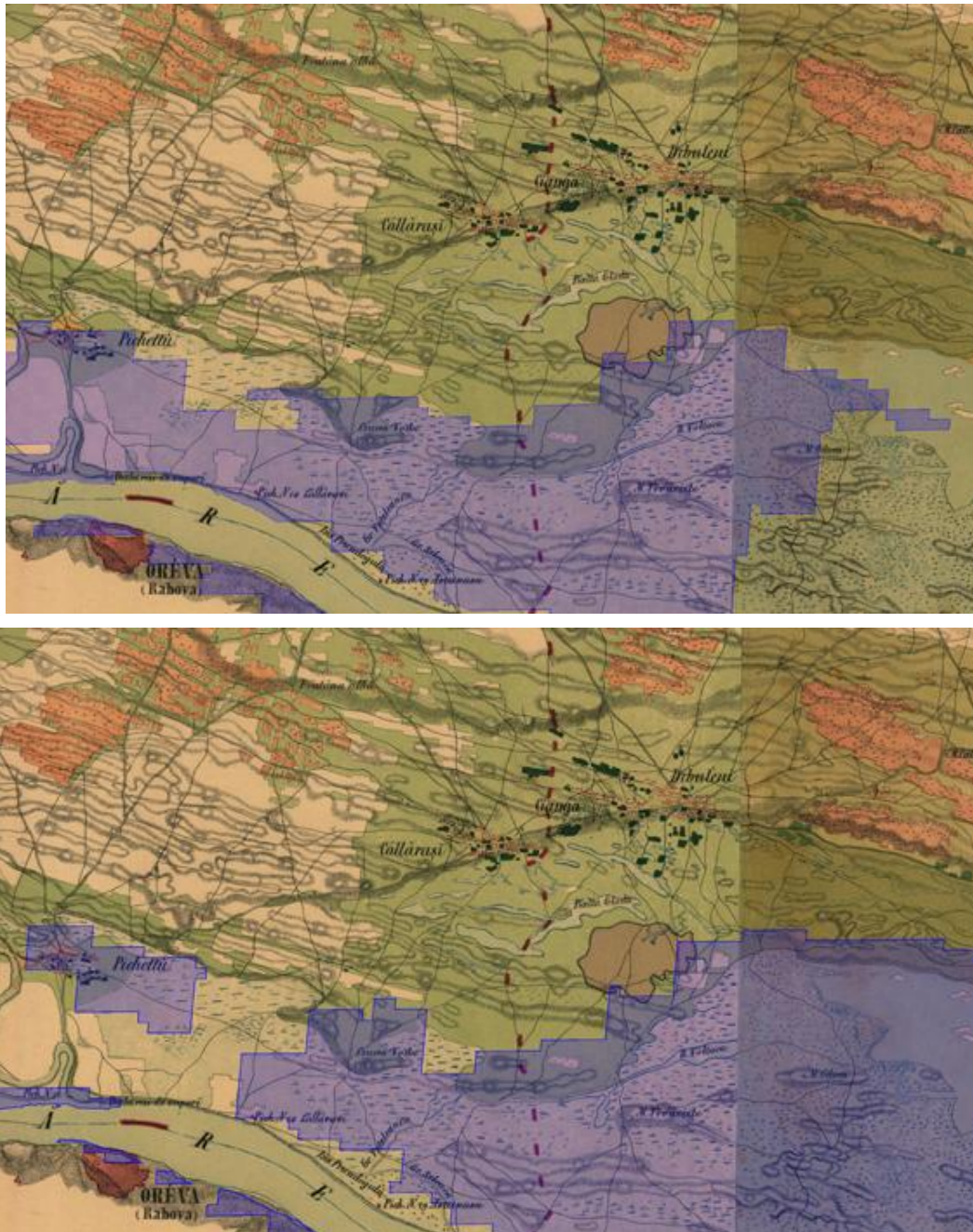
Figure 2: The 2006 flood inundation pattern on the 1864 historical map mosaic near Bechet. Note that the Danube did not reach all of the low floodplain. The extents of Figs. 1 & 2 are the same. (a) Inundation pattern of 27 April, 2006: the area on the west is inundated partly because of the banking up of a perpendicular dyke on the east, just giving through the water (b) Inundation pattern of 13 May, 2006: the old village site of Pichettu is still in an inundation pond, after the main water body left the area.
