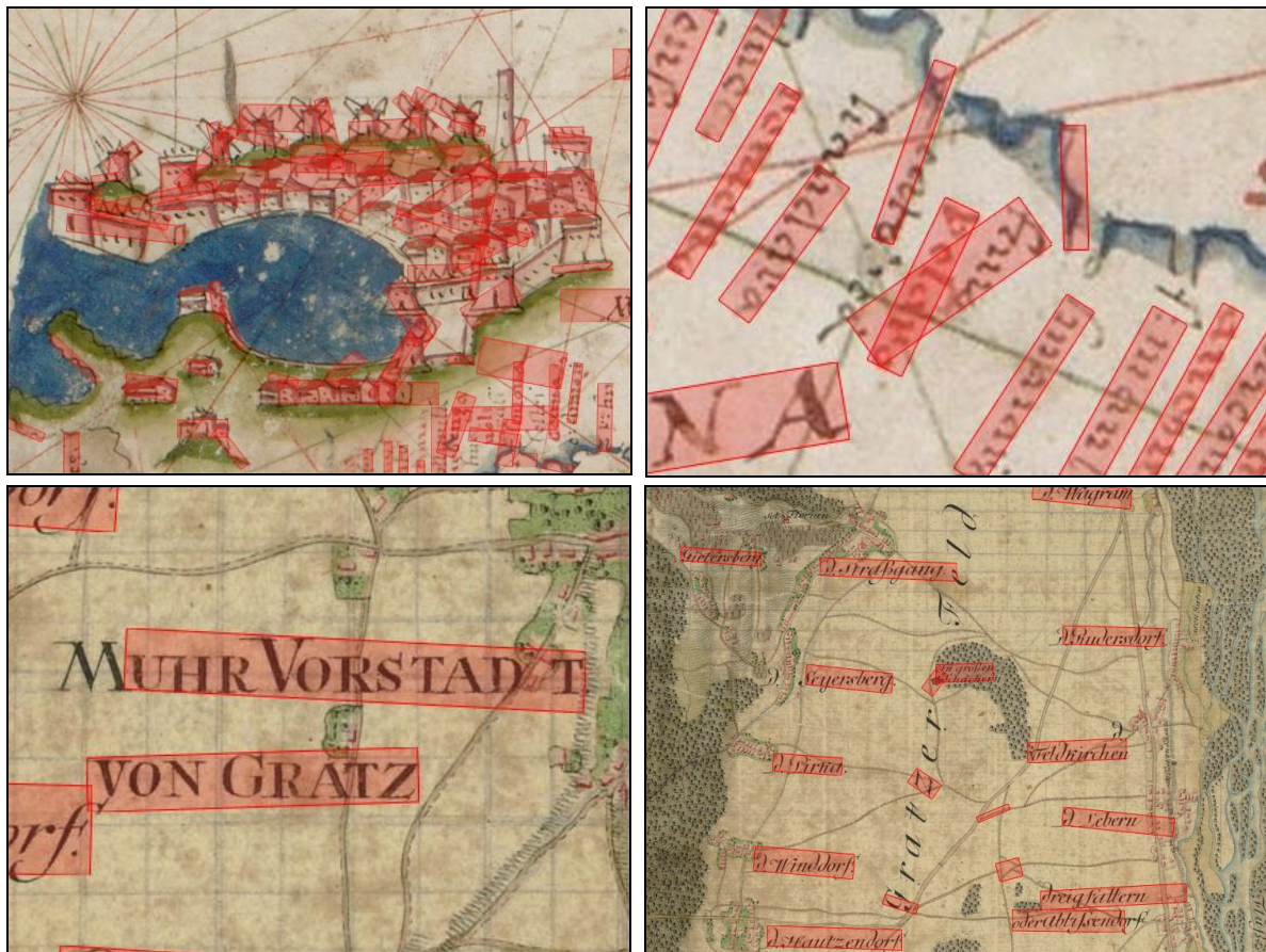
Figure 3: common error situations encountered during experiments: irritation due to symbols and ornamental features (top left); irritation due to line features flowing into toponyms, and “toponym cross-talk” (top right); split toponyms (bottom left), undetected large-area toponym (bottom right).
