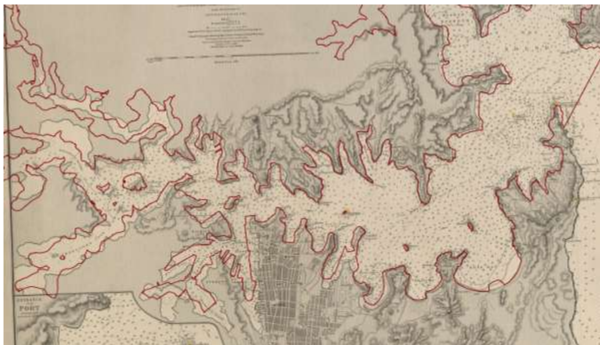
Figure 7: 1859 chart of Hutchison et al, compared with modern mean high water mark, using 22 points.
