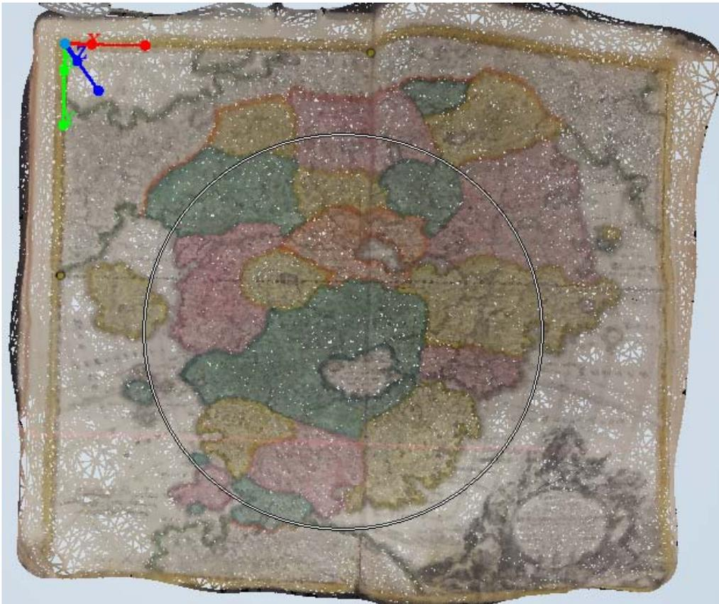
Figure 2. The Triangulated Irregular Network (TIN) after the extraction of the 3D model from 24 images of the historical map. Texture information has been applied on each point and line of the mesh.
