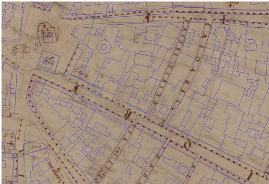
Figure 3: A detail of the overlay of the georeferenced historical map with the present numerical cartography (in blue).
