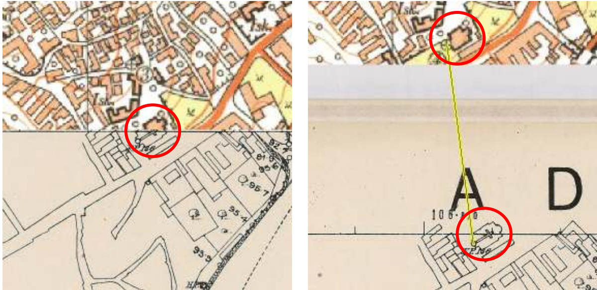
Figure 2: The error of the georeferenced map sheet: Cassini–Soldner projection (left) and stereographic projection (right)
