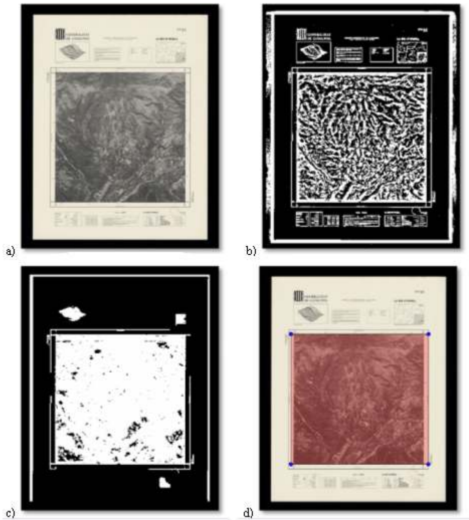
Figure 1: Map segmentation using mathematical morphology. a) Original image, b) binary image, c) filtered image after applying the morphology operators, d) original image with the bounding-box of the largest connected component.
