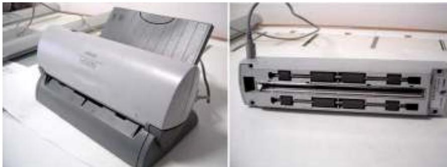
Figure 2. HS600 scanner on the ADF base (left) and rubber wheels used for movement over surface (right).
