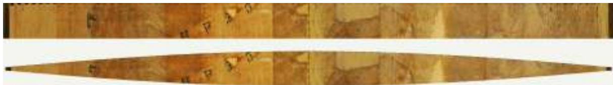
Figure 9. A Platte-Carée segment (above) transformed into Cassini's projection (below).
