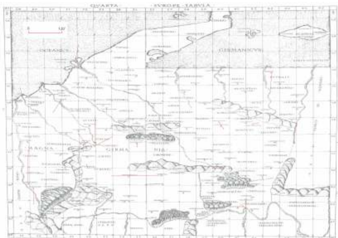
Figure 11. Displacements of toponyms (red arrows) in point-wise georeferencing of De Turre's Tabula IV to the reference map derived from coordinates given in Stevenson's edition. The displacements in the intersections of the grid traced in digital version of Tabula (green arrows) are small.
