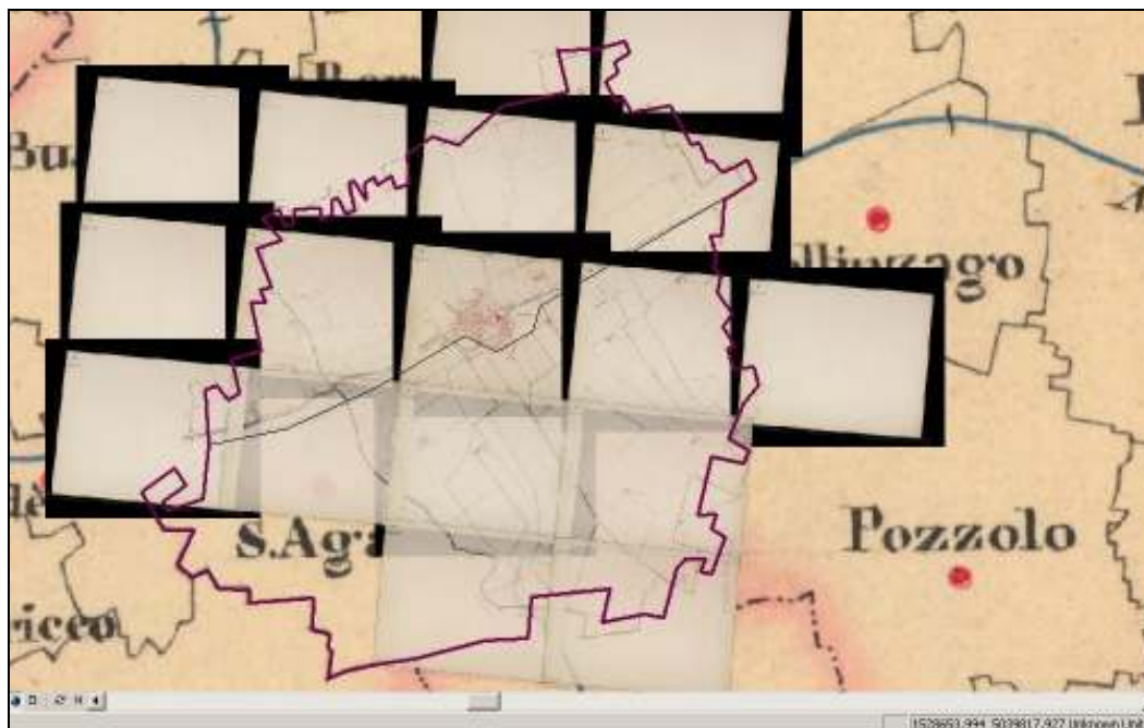
Figure 6. The overlap of the border extracted from the chorographic map and coeval border extract from the LV cadastral mosaic of the 16 georeferenced sheets of the municipality of Gorgonzola.
