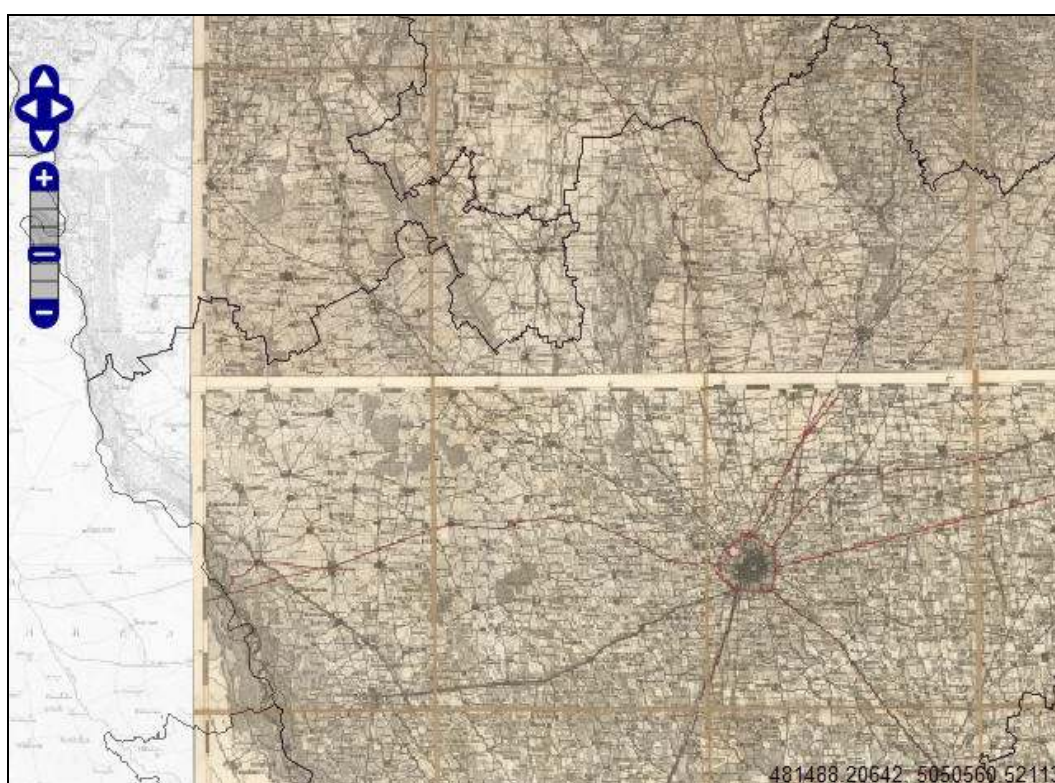
Figure 10. The two georeferenced layers superimposed on each other with respect to the current map layers: a sheet of the “Carta del Territorio del Milanese e Mantovano” (1788-1796, in scale 1:86,400), and two sheets of the same area of the “Carta del Regno Lombardo Veneto” (ITM 1933, in scale 1:86,400).
