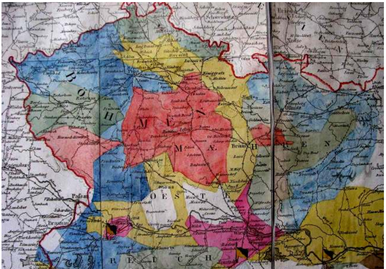
Figure 1: Military triangulation built in the former territory of Bohemia, Moravia and Silesia between 1806 and 1811. The territory triangulated in 1806 – pink, 1807 – yellow, 1808 – blue, 1810 – dark green, 1811 – red, ( Arbeiten des k. k. Generalquartiermeisterstabs... 1850 ).
