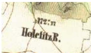
Figure 4: An example of the depiction of the spot height on the map.
