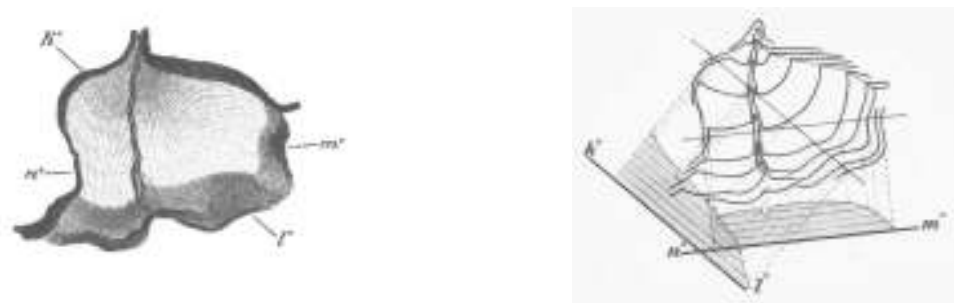
Figure 3: Landform – gully: portrayal using hachures and appropriate geometric model with depicted cutting planes and profiles ( Muster-Blätter... 1831 – 1840 ).
