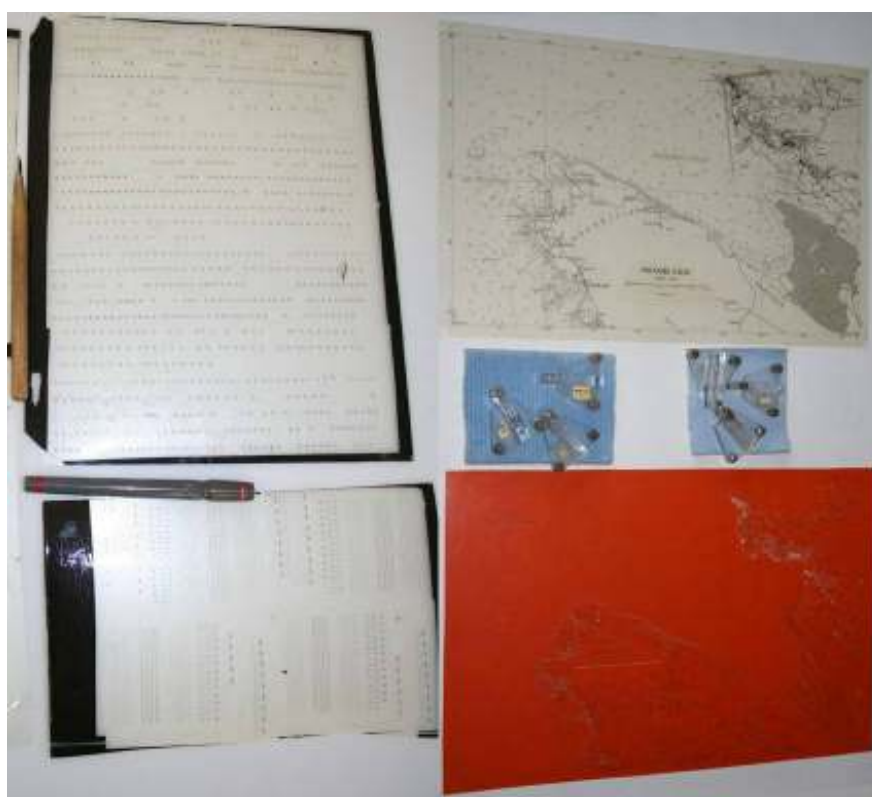
Figure 11: Old equipment for chart production: engraving pins, engraving foil, „šaber“, stripping... Part of exhibits in the cartographic section of the museum.
