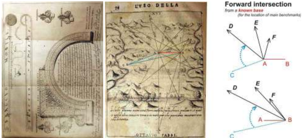
Figure 1. On left, the Squadra Mobile (mobile square) (Fabri 1673); on right, an exercise of forward intersection proposed by Fabri in his textbook.
