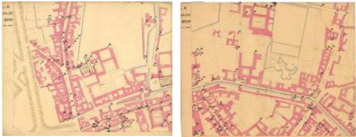
Figure 1. The sampled sheet n. 8 and 9 of the Map at the scale 1:1000 of the Astronomers of Brera, used for the accuracy test compared to the actual map at the scale 1:1000. The homologous points selected for georeferencing the two map (actual and historic ones) are evidenced in black.
