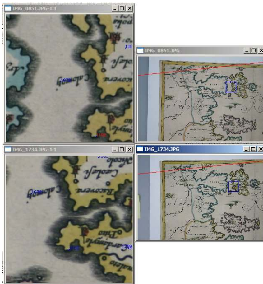
Figure 5. Matching process. The red labeled point has been extracted from the DSM generation as a bad match according to the epipolar geometry constrain.
