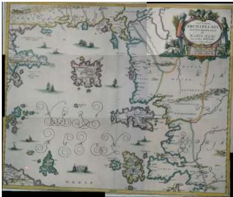
Figure 6. Final orthomosaic. No bending has been applied, on purpose, in order to distinguish the separate tiles of partial orthoimages.
