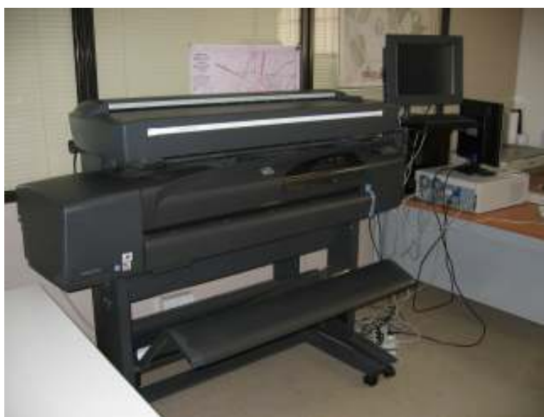
Figure 3. HP large format scanner used to scan the documents.
