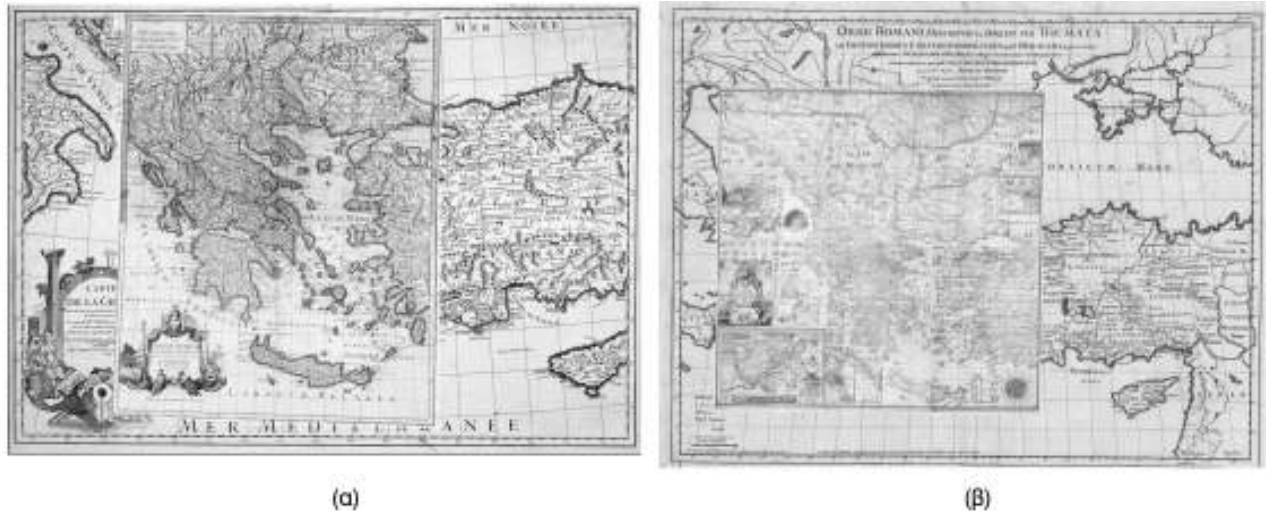
Fig. 3. α) The Delisle–A type map best fitted into Delisle–B type map. The original scale of type –A is double than that of type –B; β) Charta best fitted into Delisle–C type map. The original scale of Charta is six times bigger than that of Delisle–C type map.
