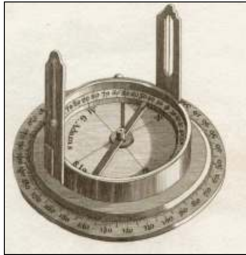
Figure 2. The simple theodolite (circumferentor) used on the Roy Military Survey.
