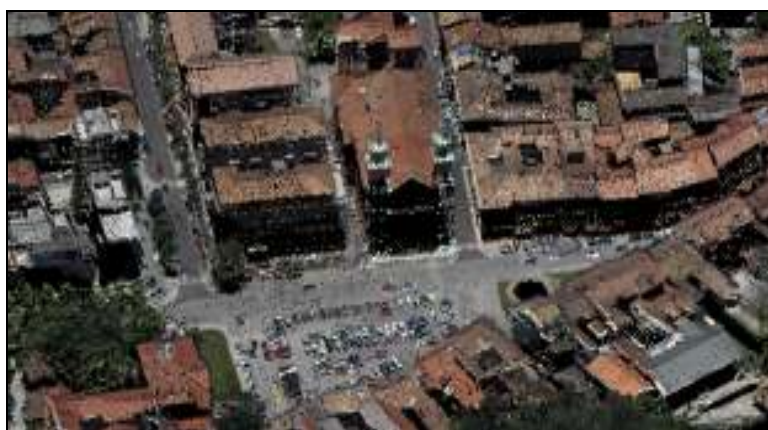
Figure 6. Laser points coloured by RGB from aerial orthophoto.
