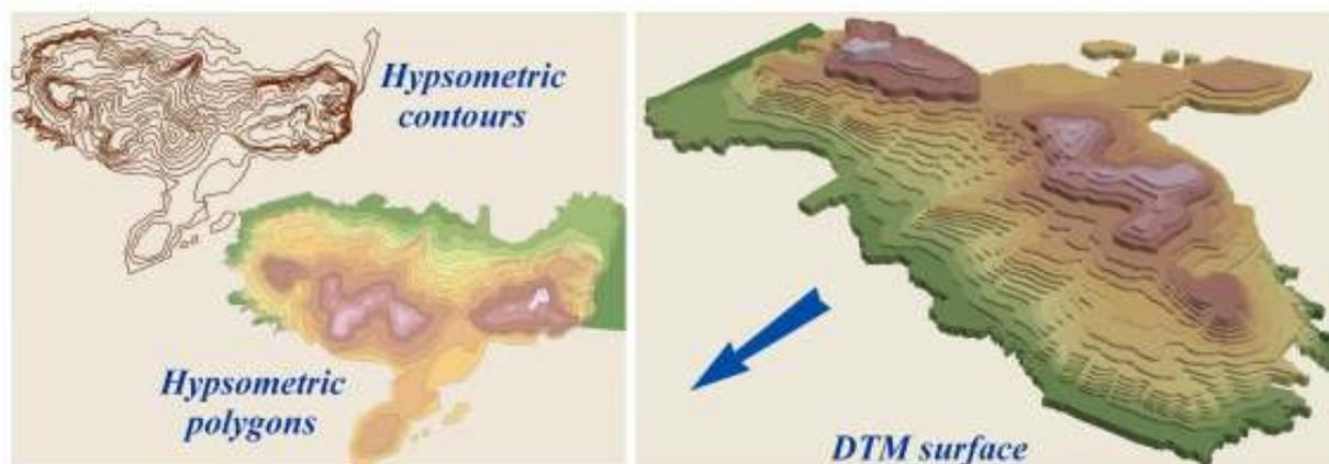
Figure 3. Creation of the Digital Terrain Model.
