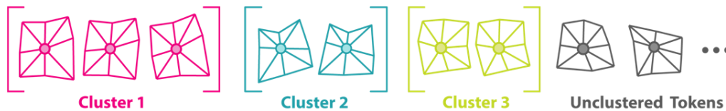
Figure 8: For every node of the deformed grid we cluster together the tokens that are similar to one another by using complete-linkage. In the figure, a possible situation is shown, where among all compared tokens three clusters were found. The tokens that are too distant to be clustered with another one are recorded as outliers, meaning that their information is not repeated in any other map.
