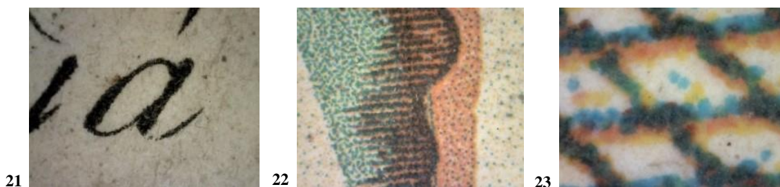
Figure 21: Photomicrograph of a printed letter produced using traditional intaglio (copperplate) printing. Figures 22, 23: Photomicrographs of blue, green, and red areas printed using offset lithography, displaying characteristic halftone dot patterns.
