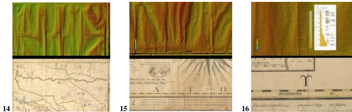
Figure 14, 15, 16: Comparative visualization using orthophotography (bottom) and Digital Elevation Models (top) of selected details from the Charta of Greece. The first two pairs of images illustrate surface undulations of the paper substrate, captured in DEM renderings through false-color elevation encoding. These variations reflect the differing hygroscopic behavior of laid paper types. The third pair reveals not only paper deformations but also traces of the printed matrix itself, offering additional insight into the mechanical aspects of the printing process. Elevation profiles along cross-sections defined in each area are metrically precise at a 1:1 scale, enabling the detailed assessment of topographic variations with high geometric accuracy.
