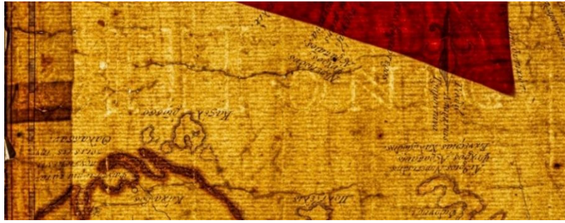
Figure 9: Transmitted light photography. The watermark “...& I Honig” is revealed through transmitted light imaging, clearly visible due to the structural transparency of the laid handmade paper.
