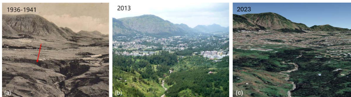
Figure 3: Landsliding area on the margin of the rapidly expanding town of Dessie with Borkena River valley in the foreground on the postcard from 1936-41, photograph by Z. Vařilová, and simulated image in Google Earth based on Pléiades satellite image from 2023. A large landslide nowadays covered by vegetation is marked by a red arrow. The vantage point is on Doro Mezleya hill (11.114600°, 39.648340°, 2540 m a.s.l.)
