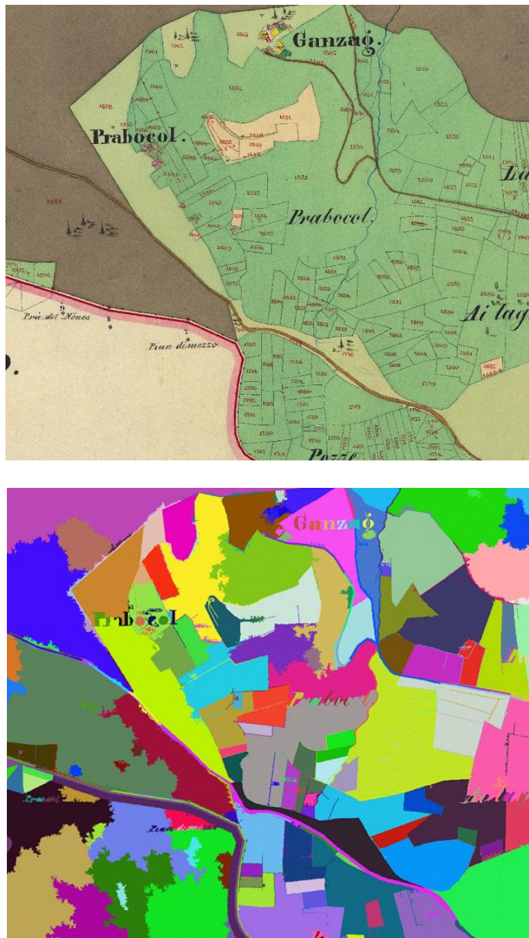
Figure 2: segmentation of the map in figure 1 with threshold equal to 0.2 and minimum size equal to 1000.
