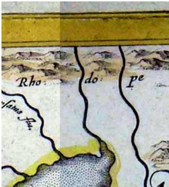
Figure 4a. The seam line between different rectified image tiles is apparent when the central projection model is used.
