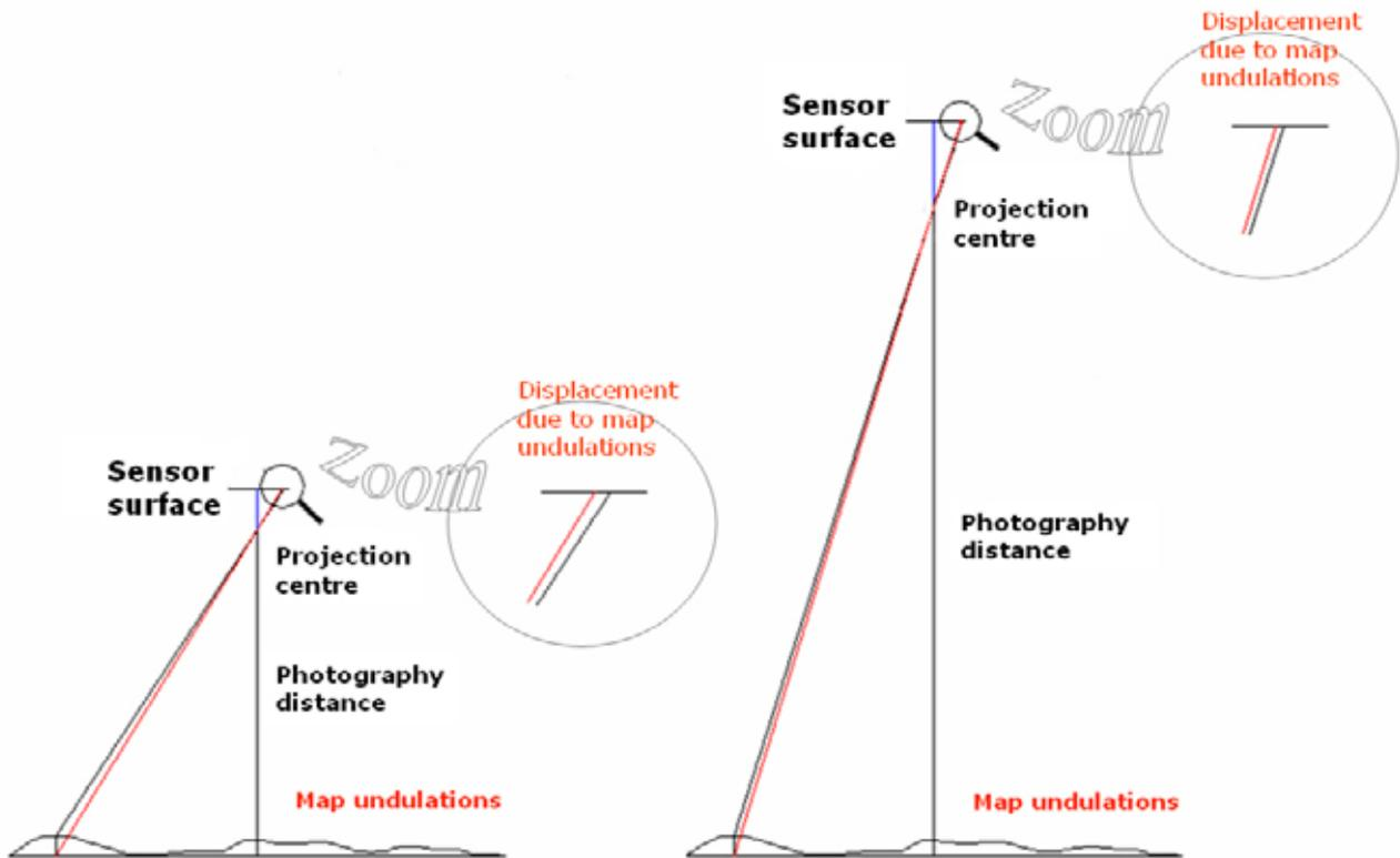
Figure 3. Displacements on the surface of the sensor due to shallow undulations on map surface. The camera constant and its distance from the object, influence the displacements.
