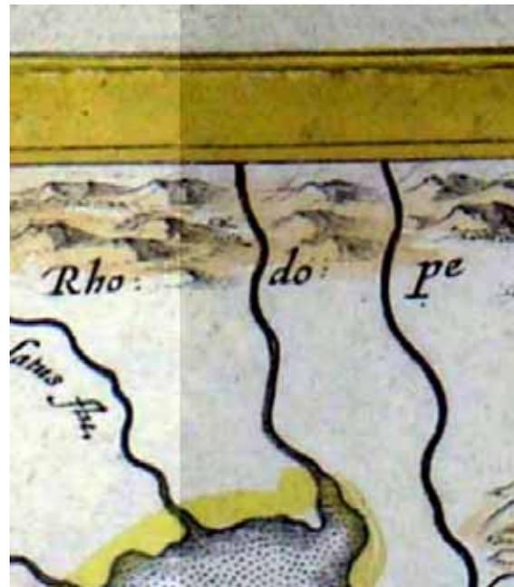
Figure 4b. The seam line is not visible when the rectification of the image is carried out using a 3<sup>rd</sup> order polynomial.
