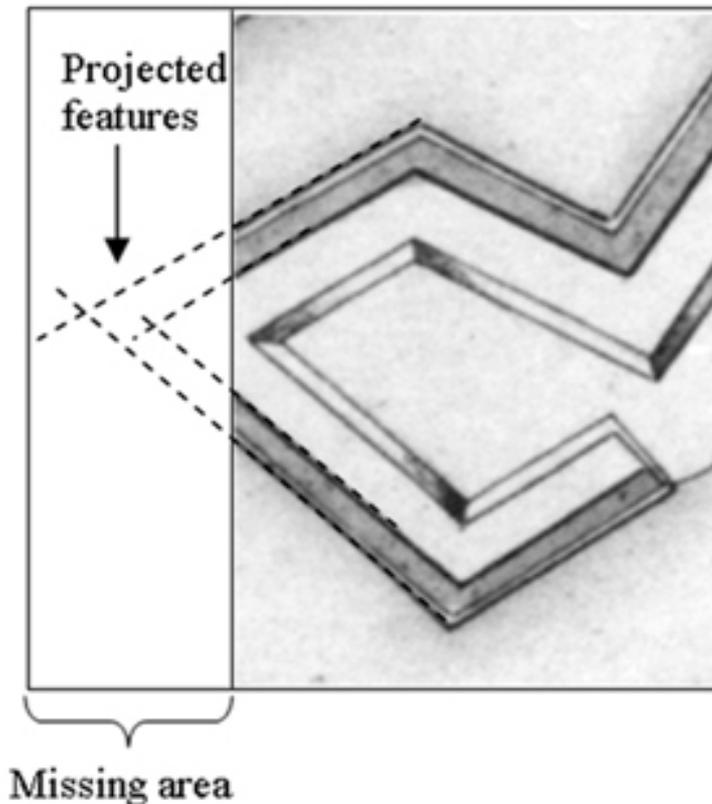
Figure 8. Bastion 8, map G35. This is an example of the case when parts of a bastion are missing due to the acquisition of the map. Here during the scanning process part of the map is cut off. The projected lines on the missed area (left) show how the shape of the bastion is reconstructed.
