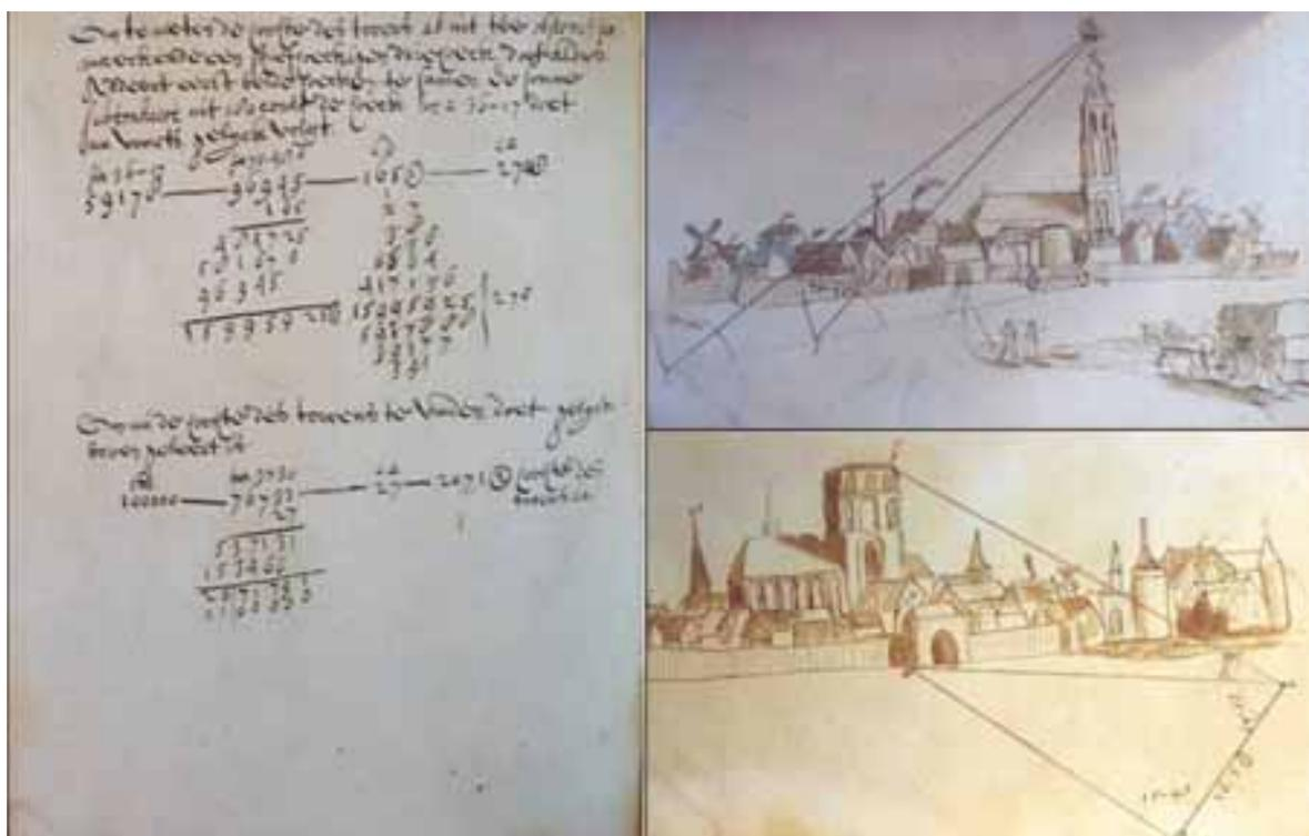
Figure 1. The measuring of angles and distances by using high spots (towers) in Zwolle.
