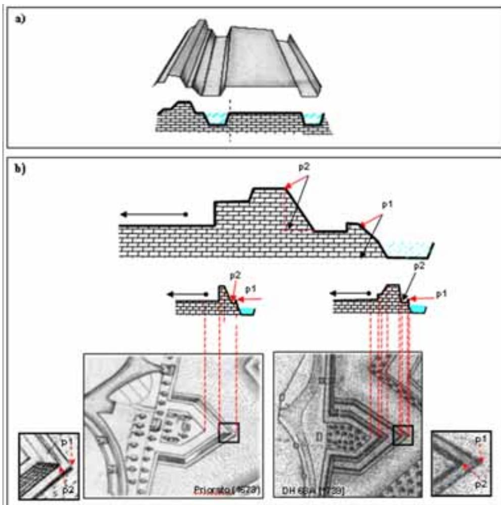
Figure 4. Profiles used for choosing common points in the historical maps of Zwolle a. Detail of a profile as on map ARA 4.OPV Z65 (1672)<sup>19</sup>. b. Detail of a bastion's profile (above) and interpretation of the profiles of the bastions depicted on the maps of Priorato (1673) and DH68A (1739) (below). The corresponding points are indicated by dotted lines.
