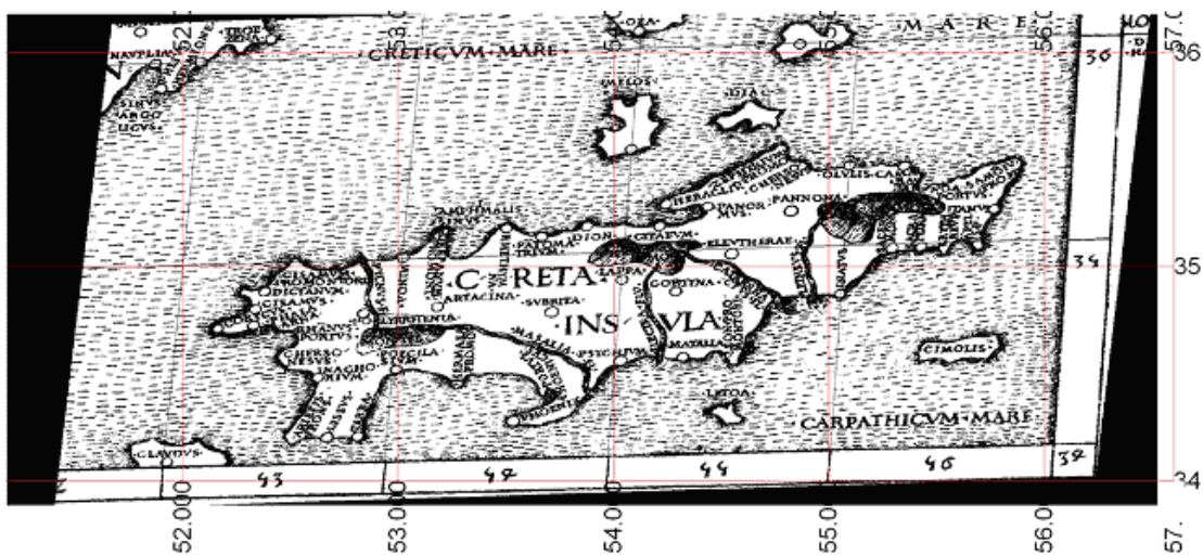
Figure 3. The calibrated map-image using geographical coordinates of ten towns on island's coastline.
