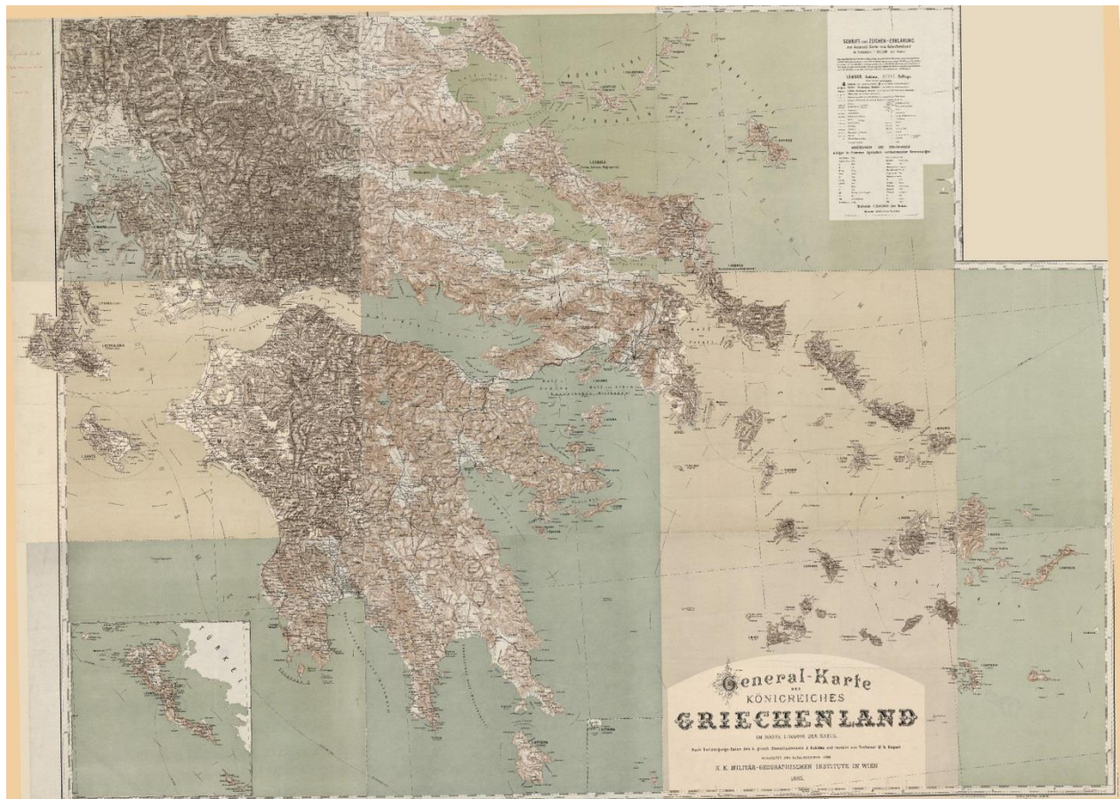
Figure 2: The Austrian 1:300,000 scale map of Greece, georeferenced in Vienna-centered Bonne projection. The exact horizontal and vertical sheet boundaries indicate the correctness of this projection.
