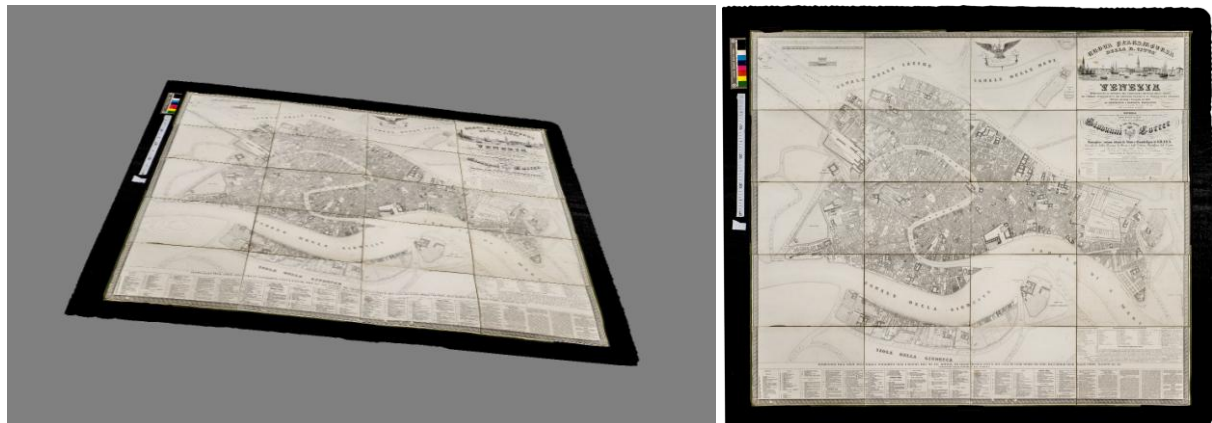
Figure 3. The Combatti map's photogrammetric model and the final orthophoto.
